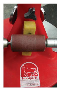
6. WHEN YOUR BUFFER SLEEVE GETS DIRT BUILDUP, SIMPLY RUN THE TOOL AND APPLY SLIGHT PRESSURE ON THE STICK. IT WILL CLEAN UP VERY QUICKLY.
