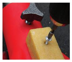
3. LAY THE HOOFJACK ON ITS SIDE, BRACE IT AND APPLY THE SELF-PIERCING SCREWS IN YOUR HOLES. MAKE SURE YOU TIGHTEN UNTIL THE HEAD IS SUNKEN INTO THE STICK ABOUT 3/4", NOT JUST FLUSH WITH THE OUTSIDE.
