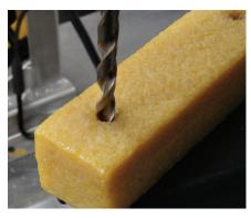
2. THE FOOTPRO RUBBER CLEANING STICKS DO NOT COME PRE-DRILLED. DRILL APPROXIMATELY HALF WAY INTO THE STICK WITH A 5/16" OR 3/8" BIT.
